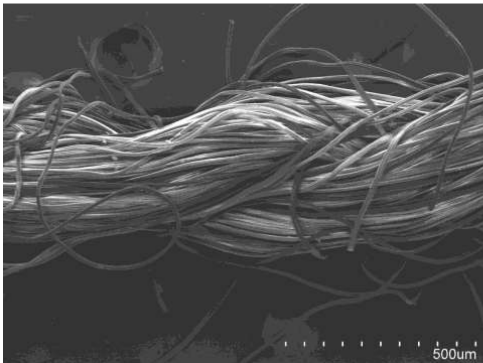
Fig. 14 (SEM) Silk Threads -Lab/4
